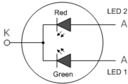
In this case we have three connections with the cathodes (K) connected in common. Either LED or both can be cut on together or alone.
