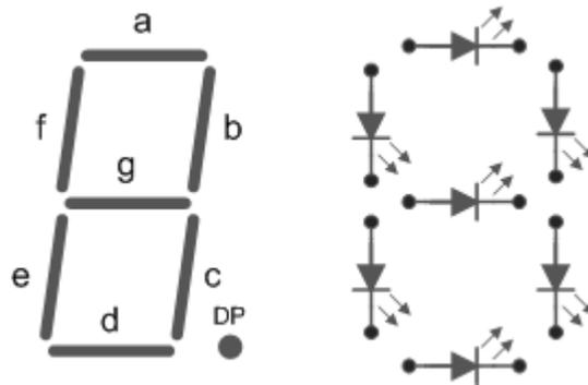
In this case we could have eight LEDs connected with a common cathodes or common anodes arranged to produce a numeric display for a calculator.
