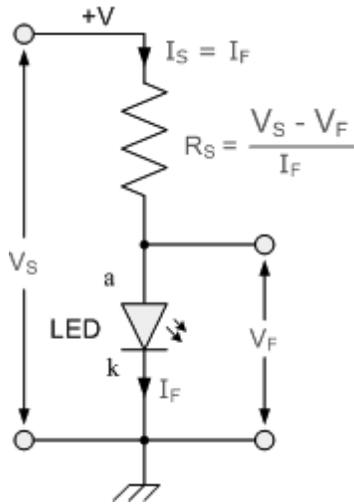
$$R_S = \frac{V_S - V_F}{I_F} = \frac{5\text{v} - 2\text{v}}{10\text{mA}} = \frac{3}{10 \times 10^{-3}} = 300\Omega$$
